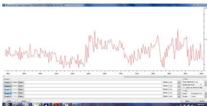
Fig.3.22: Congestion response with frame sizes between 401-800 bytes {Medium (M)}
