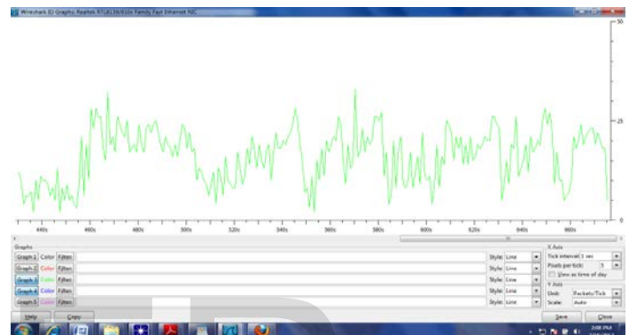
Fig.3.24: Congestion response with frame sizes greater than 1200 bytes (Extra-large (XL))
